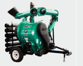
The VRX sets the standard in grain vac technology and has capacity up to 6,000 BPH. The VRX sports 45-feet of 7-inch diameter hose. Combined with the telescoping inlet and the standing floor sweep, the VRX cleans up grain within a 49-foot radius from the base of the machine.
