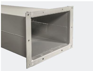
12 GA (2.75 mm) fixture welded trunking is standard on all AGI powder-coated and galvanized bucket elevators, with 10 GA (3.41 mm) trunking available on request.
