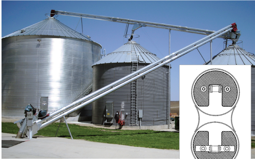
Stationary double run can be used in various applications at angles from horizontal to 60°. Lengths available in 5' increments. A flow through inlet is convenient for overhead applications.
