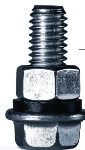
Grade 8.2 bin bolts are used throughout to ensure strengths and stability. Roofs and lighter gauge sidewalls use 5/16" (0.79 cm) bolts. Heavier gauge sidewalls use 3/8" (0.95 cm) bolts.
