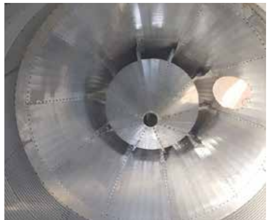
— Photo of hopper silo aeration cone mounted on silo
