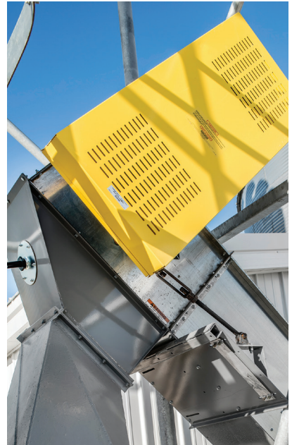
All Dodge speed reducers come furnished with a drive guard that meets OSHA standards .
